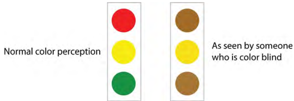
Figure 3: Traffic light colors, which are often used on dashboards, and how they are seen by most people who are color blind.
